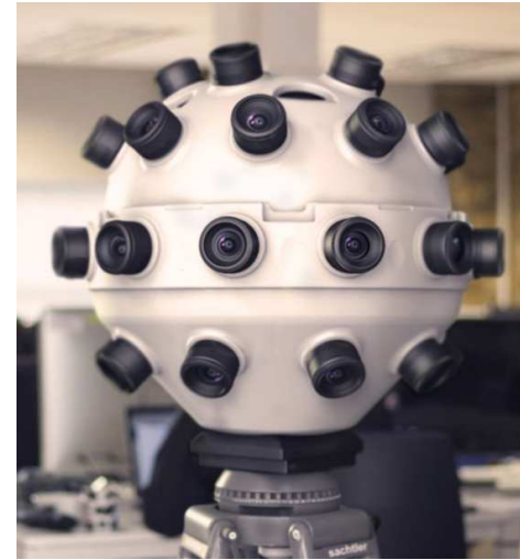
Figure 7.25: The Pantopticom prototype from Figure Digital uses dozens of cameras to improve the ability to approximate more viewpoints so that stereo viewing and parallax from position changes can be simulated.
