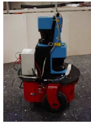
Fig. 12. Setup used to validated the gaps model. A robot was provided with two SICK lasers.
