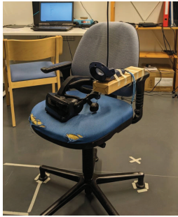
Fig. 4. Experimental setup with a rotating office chair equipped with a tracker to track the chair heading during rotation.
