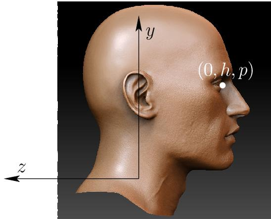
Figure 9.8: To obtain a *head model*, the rotation center is moved so that orientation changes induce a plausible translation of the eyes. The height  $h$  is along the  $y$  axis, and the protrusion  $p$  is along the  $z$  axis (which leads a negative number).
