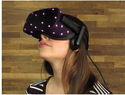
Figure 9.13: The Oculus Rift headset contains IR LEDs hidden behind IR-transparent plastic. (Photo from [www.ifixit.com](http://www.ifixit.com).)
