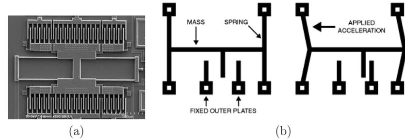
Figure 9.2: (a) A MEMS element for sensing linear acceleration (from [36]). (b) Due to linear acceleration in one direction, the plates shift and cause a change in capacitance as measured between the outer plates. (Figure by David Askew, Mouser Electronics.)
