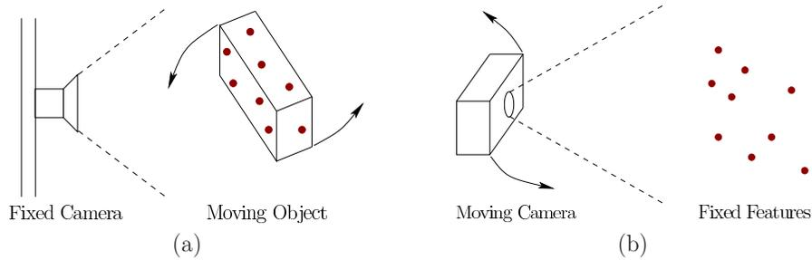
Figure 9.15: Two cases for camera placement: (a) A *world-fixed camera* is stationary, and the motions of objects relative to it are estimated using features on the objects. (b) An *object-fixed camera* is frequently under motion and features are ideally fixed to the world coordinate frame.
