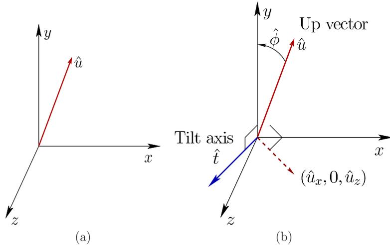
Figure 9.4: (a) Tilt error causes a discrepancy between the  $y$  axis and the sensed up vector that is rotated using the estimate  $\hat{q}[k]$  to obtain  $\hat{u}$ . (b) The *tilt axis* is normal to  $\hat{u}$ ; a rotation of  $-\hat{\phi}$  about the tilt axis would bring them into alignment, thereby eliminating the tilt error.
