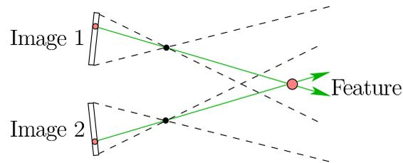
Figure 9.27: By using two cameras, *stereo vision* enables the location of a feature in the 3D world to be determined by intersecting the corresponding visibility ray from each camera. To accomplish this, the camera calibration parameters and relative poses must be known. Similarly, one camera could be replaced by a laser that illuminates the feature so that it is visible to the remaining camera. In either case, the principle is to intersect two visibility rays to obtain the result.
