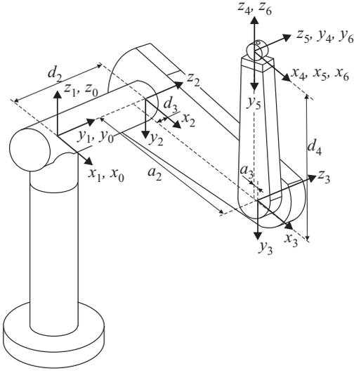
Figure 3.16: The Puma 560 is shown along with the DH parameters and body frames for each link in the chain. This figure is borrowed from [291] by courtesy of the authors.
