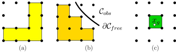
Figure 8.21: (a) An interpolation region,  $R(S)$ , is shown for a set of sample points,  $S$ . (b) The interpolation region that arises due to obstacles. (c) The interpolation region for goal points must not be empty.
