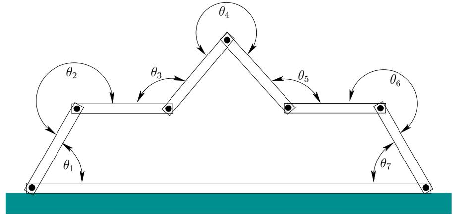
Figure 7.23: A chain of links in the plane. There are seven links and seven joints, which are constrained to form a loop. The dimension of  $\mathcal{C}$  is seven, but the dimension of  $\mathcal{C}_{clo}$  is four.
