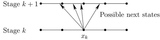
Figure 8.19: Even though  $x_k$  is a sample point, the next state,  $x_{k+1}$ , may land between sample points. For each  $u_k \in U(x_k)$ , interpolation may be needed for the resulting next state,  $x_{k+1} = f(x_k, u_k)$ .
