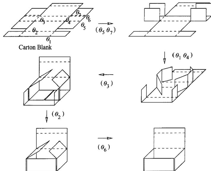
Figure 7.30: A folding sequence that was computed using the algorithm in [348].
