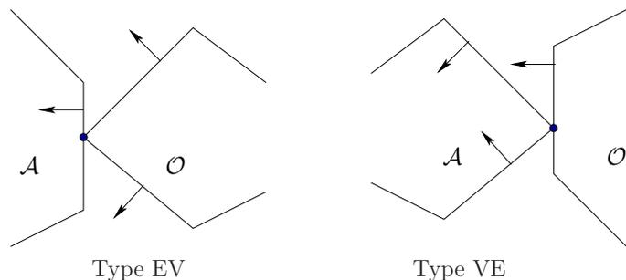
Figure 4.16: Two different types of contact, each of which generates a different kind of  $\mathcal{C}_{obs}$  edge [152, 344].
