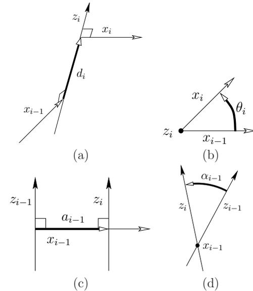
Figure 3.15: Definitions of the four DH parameters:  $d_i$ ,  $\theta_i$ ,  $a_{i-1}$ ,  $\alpha_{i-1}$ . The  $z_i$ - and  $x_{i-1}$ -axes in (b) and (d), respectively, are pointing outward. Any parameter may be positive, zero, or negative.
