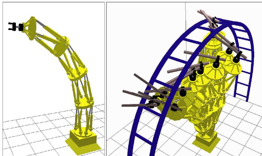
Figure 7.27: Planning for the Logabex LX4 robot [101]. This solution was computed in less than a minute by applying active-passive decomposition to an RDT-based planner [133]. In this example, the dimension of  $\mathcal{C}$  is 97 and the dimension of  $\mathcal{C}_{do}$  is 25.
