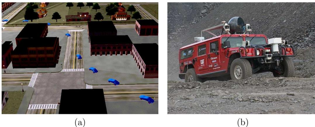
Figure 1.13: Reckless driving: (a) Using a planning algorithm to drive a car quickly through an obstacle course [199]. (b) A contender developed by the Red Team from Carnegie Mellon University in the DARPA Grand Challenge for autonomous vehicles driving at high speeds over rugged terrain (courtesy of the Red Team).
