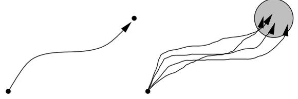
Fig. 3. [left] The robot in Example 2 gives velocity inputs that determine a nominal trajectory. [right] Nature interferes with this trajectory, but error bounds ensure that the final state is contained in a circle of radius  $t\theta_{max}$ .
