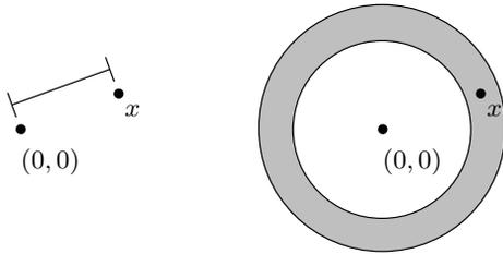
Fig. 4. [left] The robot in Example 3 has a sensor that reports a noisy estimate of the distance to the origin. [right] Accounting for noise bounded by  $\psi_{max}$ , the observation confines the robot’s state to an annulus of width  $2\psi_{max}$ .
