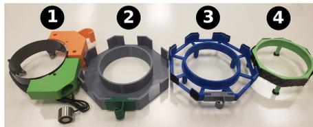
Fig. 1: Past iterations (1,2,3) and current hub design (4)
