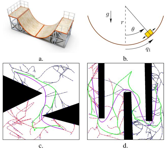
Fig. 7. a) Consider a moving vehicle on a cylindrical surface, b) the  $q_1$  coordinate behaves like an actuated pendulum, c & d) computed examples (horizontal and vertical axes correspond to  $q_1$  and  $q_2$ , respectively).
