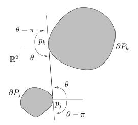
Fig. 3. An illustration of bitangent edges  $(v_j^1, v_k^1)$  and  $(v_j^2, v_k^2)$  in the nonholonomic visibility graph **G**, in which  $v_j^1 = (p_j, \theta), v_j^2 = (p_j, \theta - \pi) \in \mathbb{R}^2 \times \mathbb{S}^1$  and  $v_k^1 = (p_k, \theta), v_k^2 = (p_k, \theta - \pi) \in \mathbb{R}^2 \times \mathbb{S}^1$
