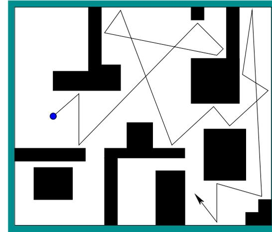
Figure 1.21: A little-brain approach implements a simple strategy of moving straight and then “bouncing” from the wall each time according to some prescribed law. One bit of memory is sufficient.
