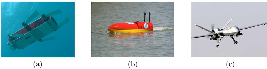
Figure 1.9: (a) The Aqua2 underwater swimming robot from McGill University. (b) A Hydronalix robotic boat. (c) The MQ9 Reaper Unmanned Aerial Vehicle (UAV).
