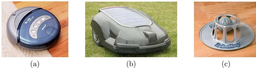
Figure 1.12: (a) A Roomba vacuum cleaner by iRobot. (b) A lawn mowing robot by Husqvarna. (c) The RoboMop floor duster.
