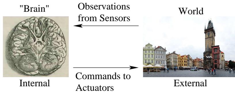
Figure 1.16: In the design of a mobile robot, we erect a boundary between internal and external realms. Information comes from the external, physical world via sensors that produce observations. Commands are transmitted to the external world that cause wheels to roll, legs to walk, and so on. The “brain” holds the information state (I-state), upon which the commands are based.
