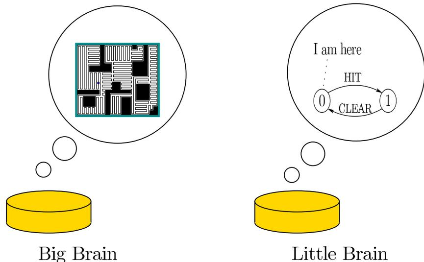
Figure 1.22: What robots are thinking. The big-brain robot maintains a full map of the environment and its own location in the map. The little-brain robot switches between only two I-states.
