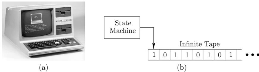
Figure 1.14: Computation models far from mobile robotics: (a) The TRS “Trash” 80, a fine example of classical computing. (b) A Turing machine, which can be imagined as a finite state machine that can read and write bits to an infinitely long tape.
