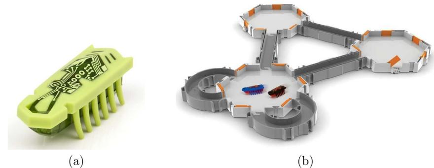
Figure 1.13: (a) A Hexbug Nano. (b) A habitat in which they can navigate along corridors and through rooms. More recent versions include one-way doors and uphill ramps that serve as escalators.
