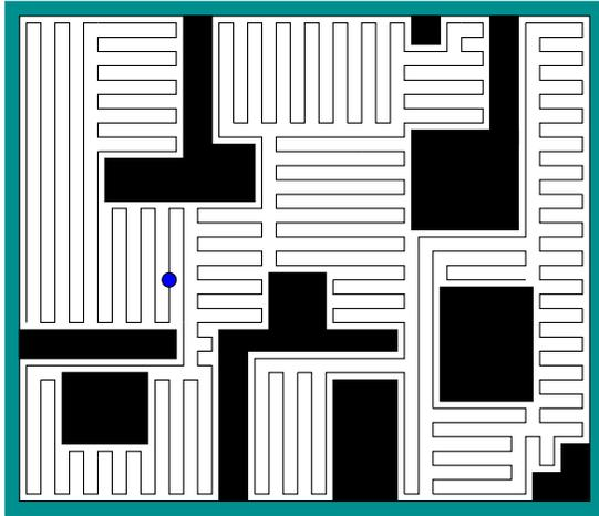
Figure 1.20: A big-brain approach to covering the whole floor area. Build a map. Determine the robot location and direction in the map. Compute a path that will complete the task. Command the robot to follow the path using powerful feedback from sensors.
