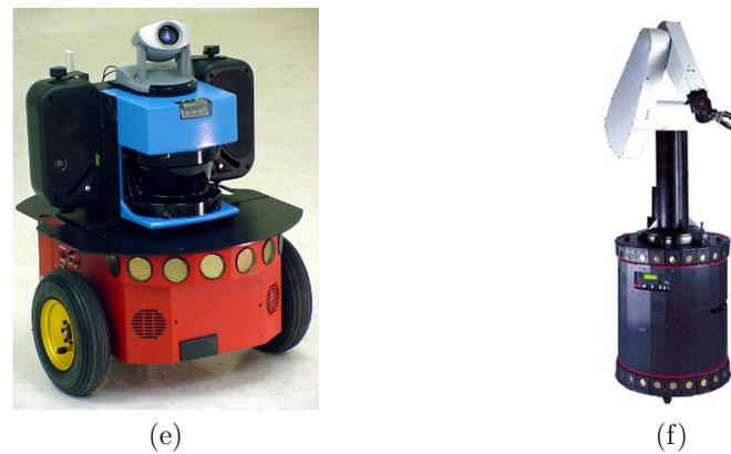
Figure 1.4: (a) Cygan the humanoid robot (1957) (b) The Stanford cart (1960s). (c) and (d) Shakey mobile robot (1966). (e) The Pioneer 3-DX8 mobile robot. (f) The Nomad XR4000 mobile robot with a Puma industrial arm mounted on top.
