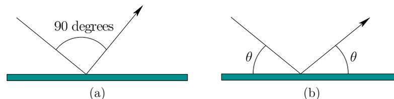
Figure 1.24: Simple, predictable rules for “bouncing” off of the wall: (a) Right angle bounce. (b) Specular reflection (as in light rays hitting a mirror).
