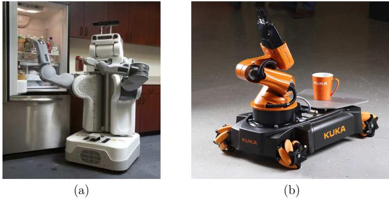
Figure 1.8: Mobile manipulators: (a) The PR2 from Willow Garage. (b) The Kuka Youbot.
