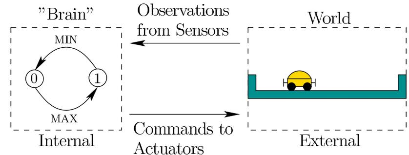
Figure 1.17: Compare to Figure 1.16. The external world is reduced to a robot that rolls along a track, capable of moving only from side to side. On each side is an independent mechanical bumper that senses whether the end of the track has been hit. A “bit brain” that solves the task of patrolling back and forth is merely a two-state machine (also called an automaton).
