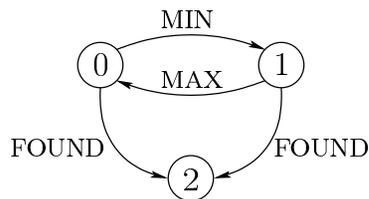
Figure 1.18: To solve a searching problem, a new I-state is added and a sensor that detects whether the spot has been FOUND.
