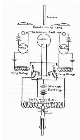
Figure 1.3: Circuit diagram of Hammond and Miessner’s 1912 electric dog.
